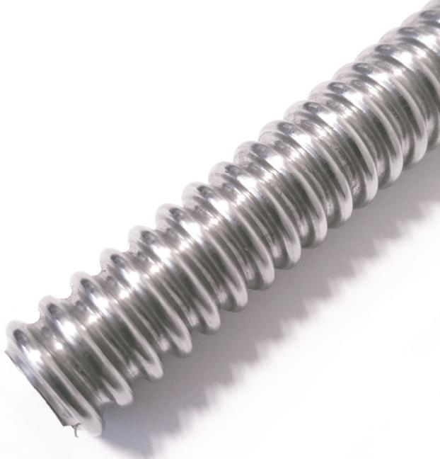
mechanically shaped corrugated hose with wide pitch corrugation, applicable under extreme conditions (-270 °C to 600°C), without natural aging, available without braid. The production method guarantees high leak tightness. Design and type approval in accordance with EN ISO 10380 standard
